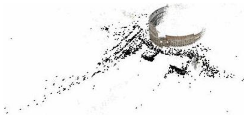
Figure 2.1: Reconstruction from 3 million images from Flickr.com . Cluster of 250 computers, 24 hours of computation. Paper: Building Rome in a Day , ICCV’09
